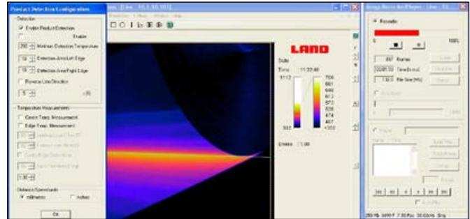
Figure 6. Thermal image of strip joining the coil.
