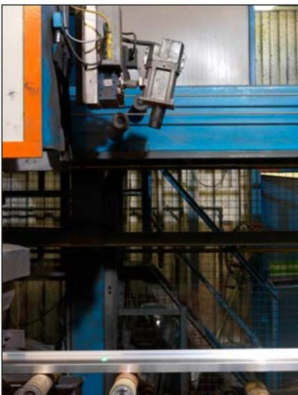
Figure 2. A pyrometer positioned at a slight angle to avoid reflections on profiles as they exit the quench area.
