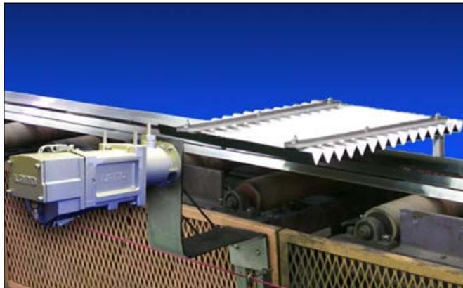
Figure 3. Reflection sources can be blocked with a radiation shield to prevent reflection effects.
