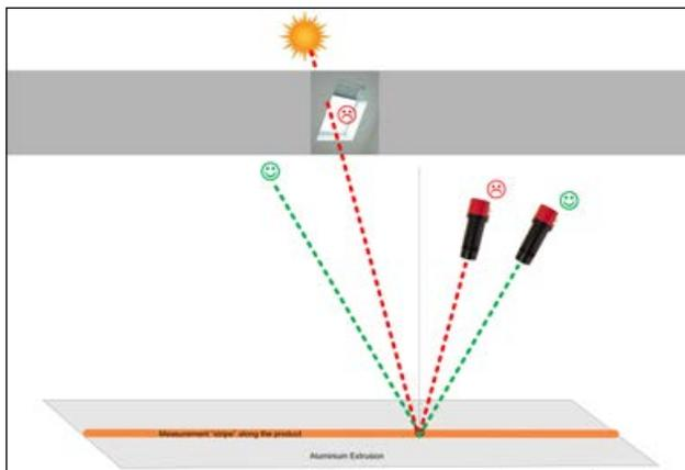
Figure 1. By understanding where reflections come from, a pyrometer can be aligned to avoid them.
