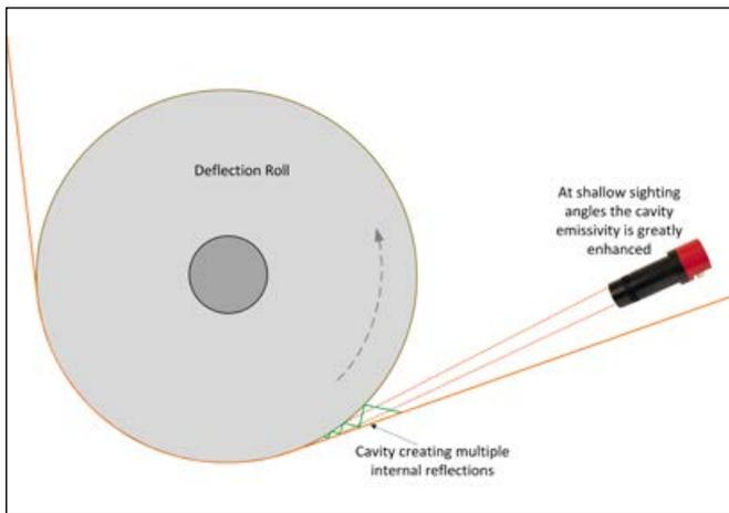
Figure 4. Pyrometer sighted into the high emissivity wedge formed by the strip contacting a roll.
